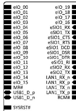
The eDNP/8331 is a "virtual" system-on-module, which can be integrated as an Altium snippet into own schematics and PCB layouts.
