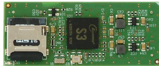
The DNP/8331 is the real system-on-module, which is available for evaluation, fast prototyping and low-volume productions.
