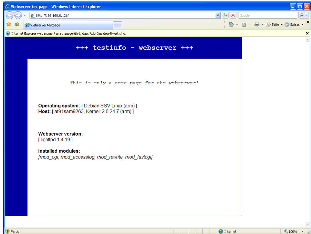
Figure 20: Checking the Web server of the IGW/963 with a browser
