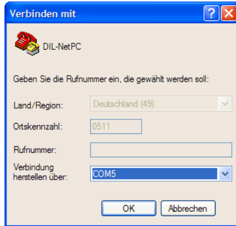
Figure 7: Direct connection setup with HyperTerminal
